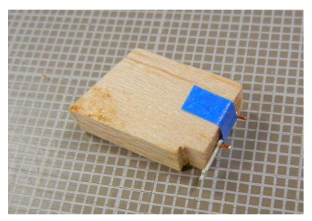
4. (DSCN0344) Drill the holes for the rails posts. I located mine by placing tracing paper over the plans, drawing in the post locations, then transferred them to the actual part. This gave me accurate locations.
