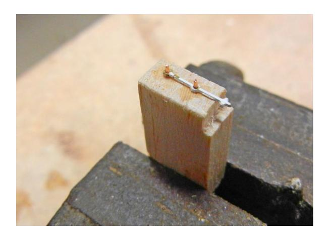
3. (DSCN0358) Install a rail on the pins and secure it in place with tape. The post is now ready to install. The tape will have to be replaced quite often for secure fastening.
