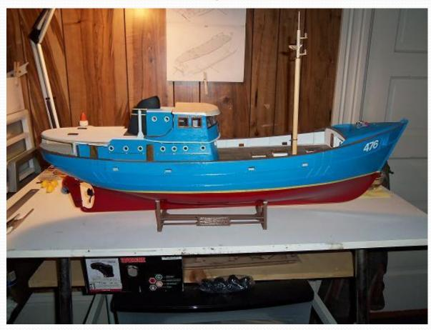
I placed (not glued) the mast to review the look. I'll paint before installing permanently.
