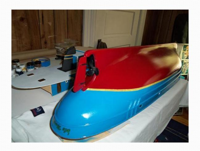
Applied the decals, painted the water line, and installed the rudder & propeller.
