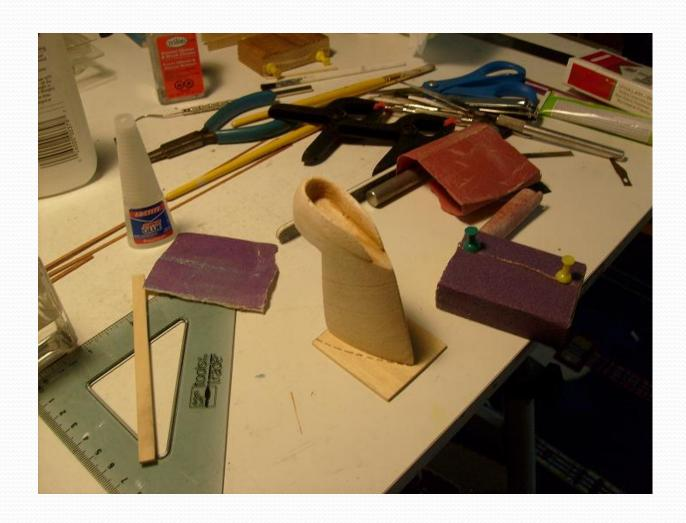
The funnel was constructed bending the wood according to the directions. Lots of sanding and smoothing.
