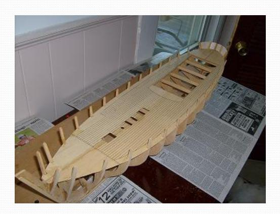
The decking mounted to the bulkheads was done prior to planking.
