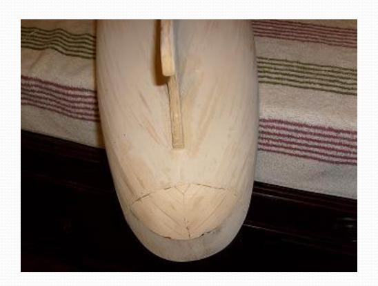
This photo shows the planking after wood filler has been applied, allowed to dry, and a "first" sand. The view also shows the stern panels installed.
