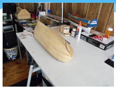
\*Soon, it was finished. I added some filler to a few of the more noticeable gaps. By the time I do the first sanding, it should be completely dry. Later, it will get a thin coat of filler, to be sanded yet again, in an effort to fill in all the cracks in the hull. First sanding will be a rough sanding, followed with a go-over with finer paper. It will be nice to feel a smooth hull.
