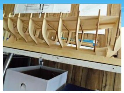
\* You may note the brads in the deck surface. I like to pull them out later, after it is dry......they are not needed anymore and it will insure that the deck planking will be flat, with no bumps. This was set aside to dry thoroughly before the next step..... fairing and hull planking.
