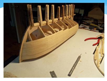
\* As the planking progressed, I noticed that the bow was coming out rather well. The stern however, was taking on the opposite results. Rather than rip boards up and waste them, I decided to simply repair the bad spots and follow it up later with filler, sanding and shaping it to the desired shape.
