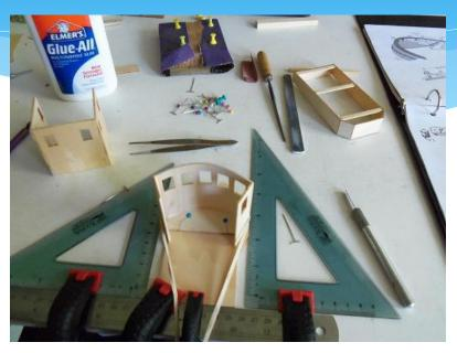
\* The face of the pilot house needs to make a significant bend here. I found the face to be made of a very stiff plywood, making this bend quite hard to do. I will replicate the part using a softer, more flexible material. I have some basswood 1/16" x 4" 24". Checking this out, I found it to be perfect for the job.
