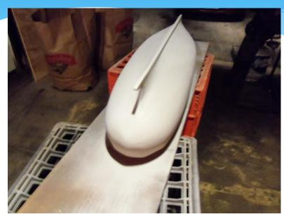
\*After the sanding was finished, the hull was given a primer coat. I find this to be a good way to see any defects and abnormalities. There were a few cracks where the glue didn't seal between the planks <but> these were all minor.....and I was quite happy with the results.
