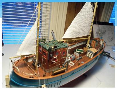
\* One by one they were threaded through the sail and the mast hoop eyelet, until they were all strung. In this last picture, you will see another line that starts {tied} to the top corner of the sail, goes through a block {that I had to add}, and goes through all of the mast hoop eyelets, and is tied off at the cleat near the base of the mast
