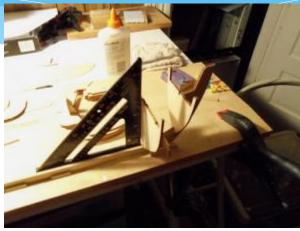
Everything was laid out and ready......so, the build began. Using my carpenter's square, the ribs were assembled onto the keel. According to the plans, pre-measured pieces of wood was cemented in between the ribs, spacing them out and locking them into position.
