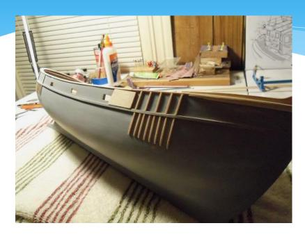
\* The rub rails were installed, sanded and cleaned up. The scupper covers were installed.
