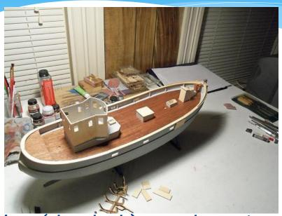
\* It (the deck) was then given the second coat (of lacquer)..when that was dry, the structures were set on it for a dry fitting to see how it would look.
