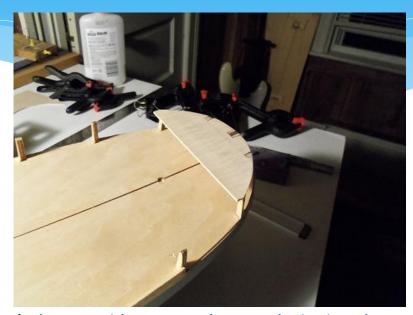
\* Then, an idea came about redesigning the aft deck..... I liked it......it's going to add so much to the build! The first thing to note was the shape of the deck. To do what I wanted to do, it needs to be a bit bigger, so I will extend it to the 9th pair of posts....not too much. I will raise it to the top of the posts and add a wall in the front
