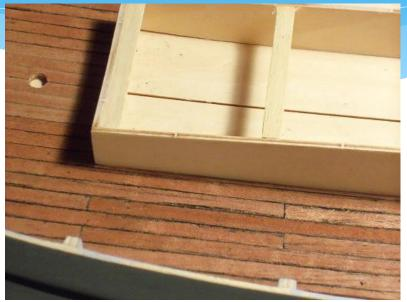
\* I used small strips of planking to space the leading rows. Black crayon outlines the outer edges of the planks to simulate caulking. Excess is scraped off the top surface and assembled into a pile on the table, along with sanding dust from sizing the planks. It is mixed together and used to fill in any small gaps in the deck.
