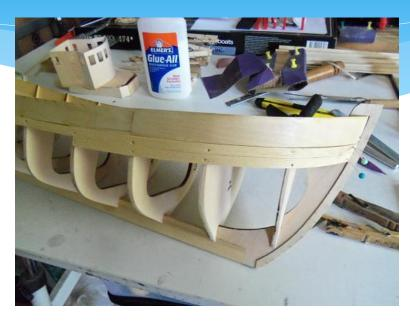
\* Planking the hull was the next step in the assembly. The first couple rows of planking was straight forward, not too much to worry about.
