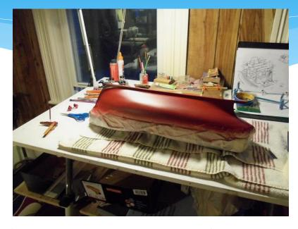
\* I am going to paint the bottom first... makes masking easier. The Billing's paint ran very well through the airbrush! I did thin it down a bit, even though the paint looks quite watery. The coverage is very good......no splatter, no sputter....except when you begin to run out! I have to use a 1/4 oz bottle with this airbrush, so it does empty out quickly. I went through almost the entire 1/2 oz bottle of Hull Red. I gave it two coats.
