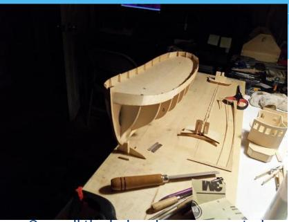
Once all the bulwarks are cemented into place, set the assembly aside for it to dry completely, before starting the hull planking. At a later time, the top of the bulwarks can be sanded level and flush with the post, for when it is time to install the top rails.
