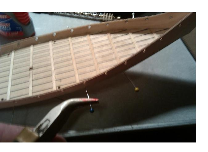
Carefully glue the sideboards to the boat. The sideboards should be closely molded to the boat already, so gluing should be relatively easy. Use pins at regular intervals to help hold the sideboards to the deck while the glue drying.
