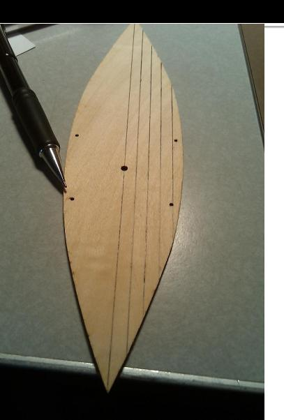
Draw parallel lines on the deck of boat this will simulate the planking. Start at the center line and work towards the sides.
