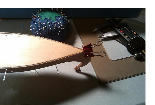
Attach shield to the side of the ship using the holes that can be seen here on the sideboards.
